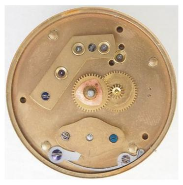
Markings on the barrel bridge of movements made in August and later have a new style which became the standard AT&Co appearance till the mid-1860s. See <u>AT data sheet</u>. Here is movement view for AT #5190 (permission of owner).
