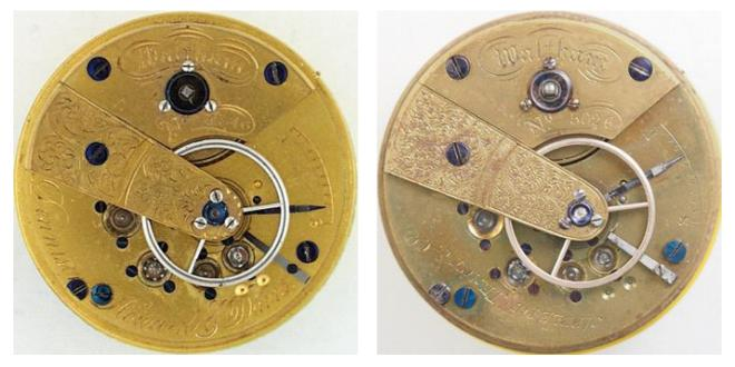
By observed surviving watches from the new company, it looks like the first 100 movements were exact DH&D copies except for the name AT&Co (AT). Robbins produced these movements starting in July of 1857. First number is 5001. View of AT #5026 movement is on the right. Markings on barrel bridge still the same, facing center; new signature facing center instead the edge. Everything inside still the same.
