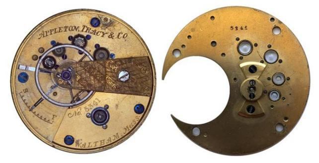
The time period "fairly quickly" is relative because there were not enough parts other than frames like wheels, jewels and escapements that had to be made to complete 1,170 movements. Nevertheless, the large number of leftover frames is significant, especially because they consist of top and bottom plates with their attached parts.
