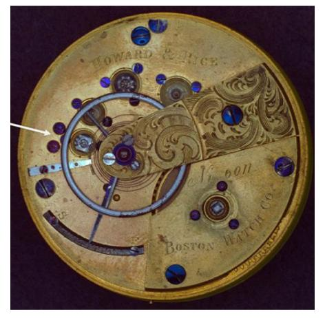
Note, for example, the two screw-adjustable banking pins which the DH&D movements did not have. Howard cannibalized seized DH&D movements and parts from the bankrupted company to make these movements.
