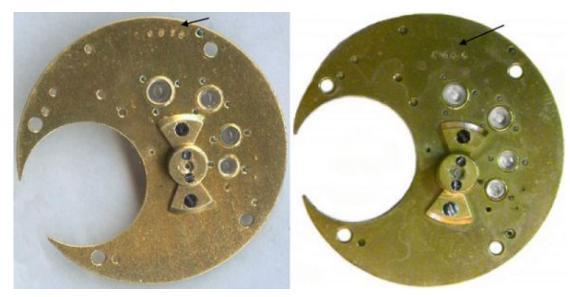
The potance supports the bottom balance arbor. DH&D on left, AT on right.
