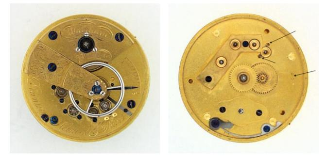
There were minor differences in the movements as the production evolved over time. The differences are documented in my monograph. For example, there are 2 "peep holes" on the latter pillar plate in which to see the escapement in action that the early versions did not have. Also note sub-assembly number 46. The steel wind guard was added around S/N 1600.
